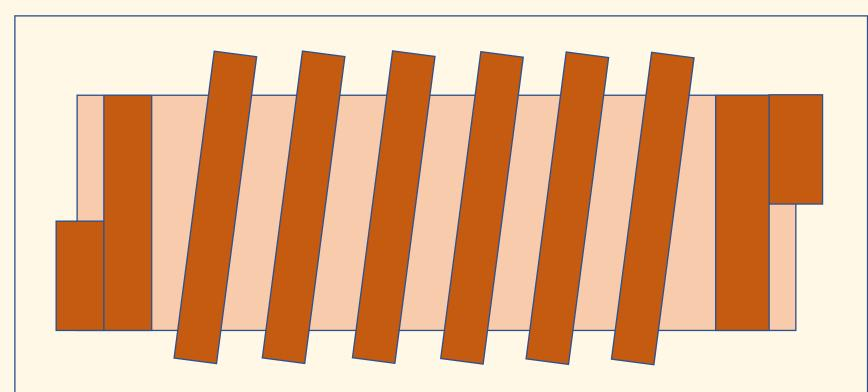
Example Sketch of Panel showing underside interlocking construction Nominal overall area per panel 1500mm \* 500mm = 0.75sq.m.
